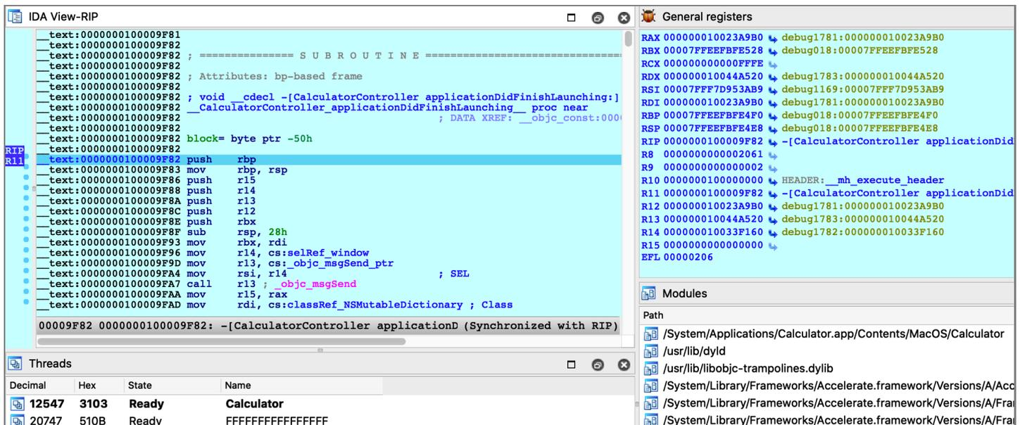
The effects of SIP are also apparent when attaching to an existing process. Try using menu **Debugger>Attach to process**, with SIP enabled there will likely only be a handful of apps that IDA can debug:
