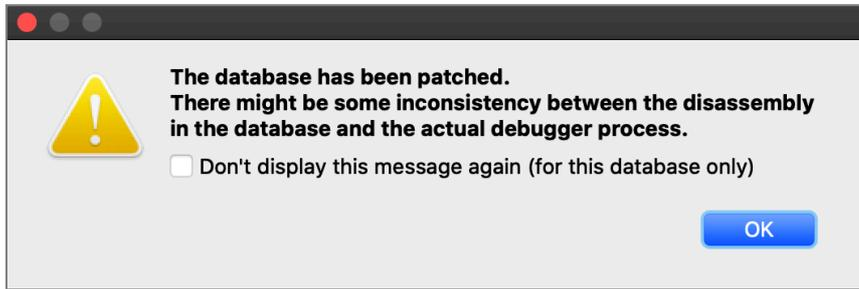
This is normal. Modules from the `dyld_shared_cache` will contain tagged pointers, and IDA patched the pointers when loading the file so that analysis would not be hindered by the tags. IDA is warning us that the patches might cause a discrepancy between the database and the process, but in this case we know it's ok. Check **Don't display this message again** and don't worry about it.
