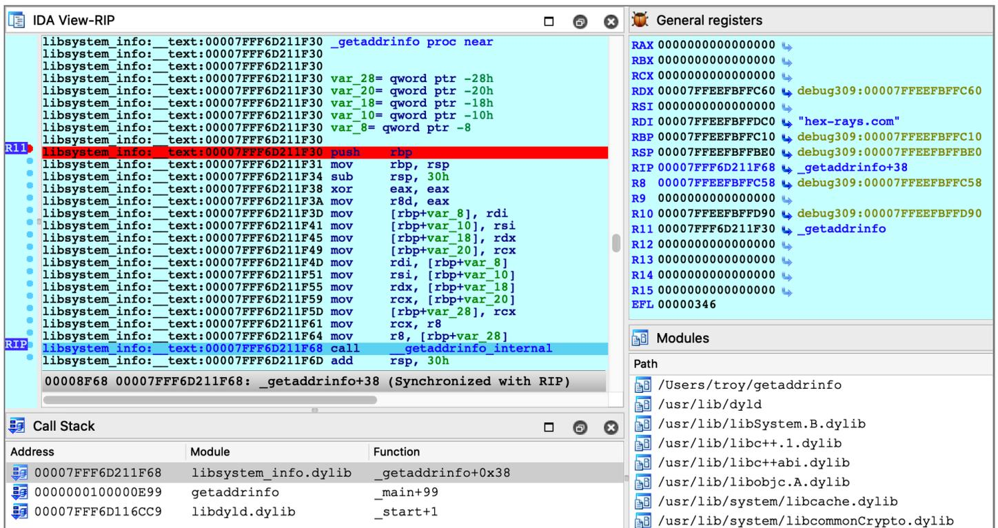
This time there was no special logic to map the database into process memory. Since we loaded the module directly from the cache, segment mappings already match what's expected in the process. Thus only one rebasing operation was required (as apposed to the segment scattering discussed in the previous example).
