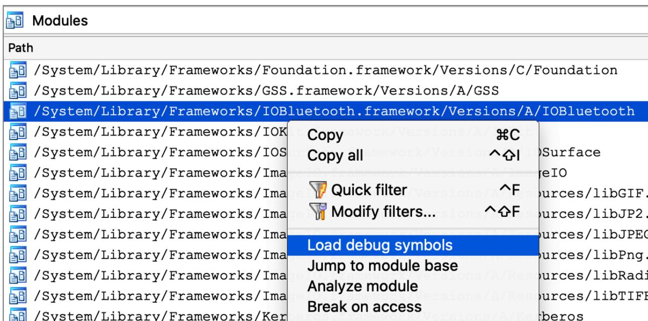
This operation will extract any Objective-C types encoded in the module, which should give us some nice prototypes for the methods we're stepping in:
