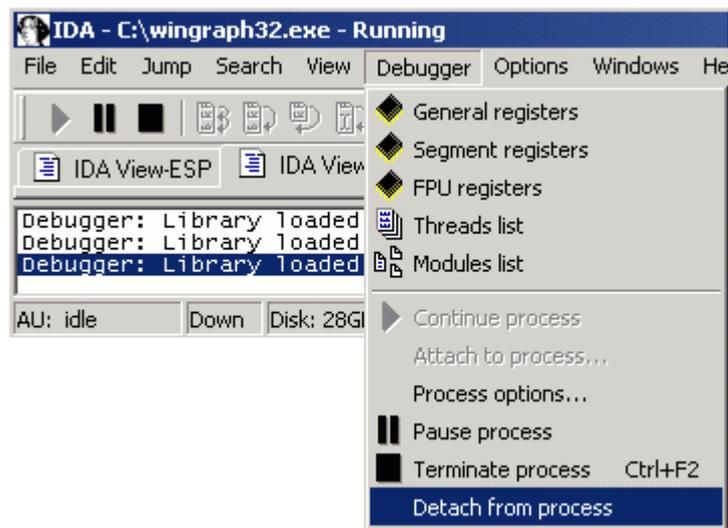
IDA supports debugging of DLLs on Windows and shared libraries on Linux. On Windows, please note that IDA can also attach to Windows services running either locally or remotely. In particular, the '*Detach from process*' command will be especially useful if you previously attached to a Windows service: it will allow you to stop the debugger without terminating a critical Windows service on the debugger server!
