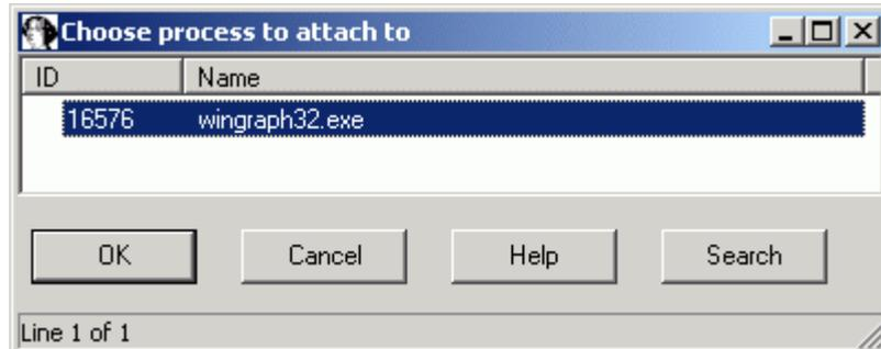
Double clicking on a process from the list will automatically suspend the process and attach to it, allowing you to debug it without starting it manually. This attach process works from Windows to Linux, from Windows to Windows, from Linux to Linux and from Linux to Windows.
