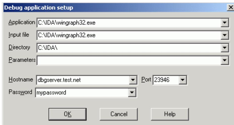
Specify the *Application*, *Directory* and *Input file* paths. Note that these file paths should be valid on the remote debugger server. Also do not forget to enter the host name or IP address of the debugger server: remote debugging will only be enabled if these settings are specified ! Finally, we enter the password we chose for the remote IDA debugger server.
